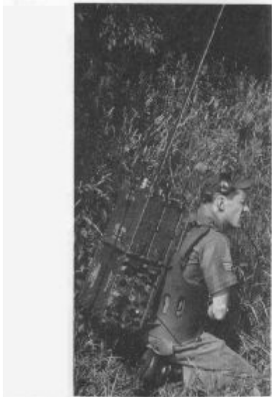
AN/PRC-71 (1965) FOUR INDIVIDUALLY PACKAGED BATTERY-OPERATED TRANSCEIVERS USED BY FORWARD AIR CONTROLLERS
