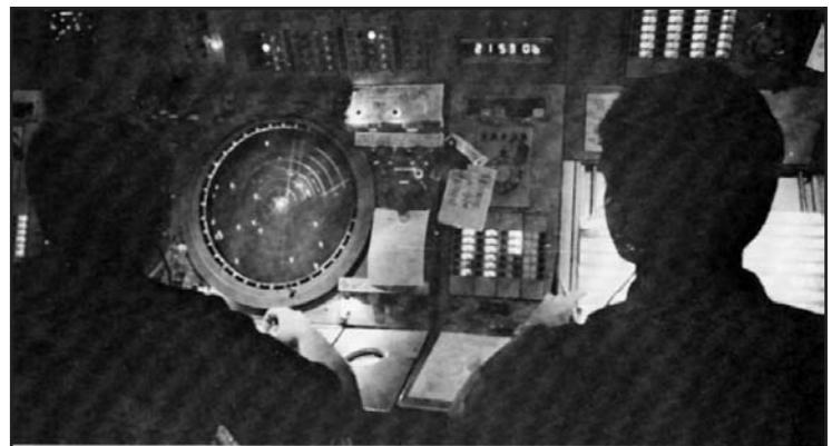
Controllers at stations in Grissom's RAPCON. "Blips" on radar screen are aircraft in 3,000-square-mile air space controlled by base. Aircraft in air space that do not contact RAPCON present potential danger to other aircraft.
