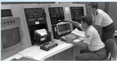
An AFSATCOM programmer, TSgt Otis Smith, operates the AFSATCOM simulator while 2nd Lt Rick Mahoney, test analyst, watches. The simulator can reproduce the inputs and outputs that show real-world choices that can be handled by radio receiver, transmitter, and satellite equipment. Tinker AFB, OK, 1983.
