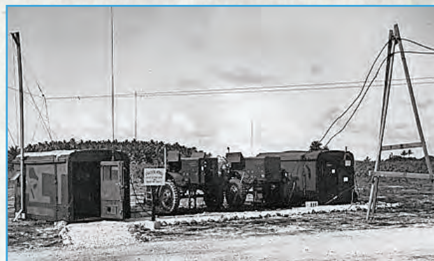
AN/GRC-26 Radio vans provided communications and MB-5 power units provided power for the island, Penrhyn Atoll. (Courtesy 6th Weather Sq (Mobile) Alumni Association)
