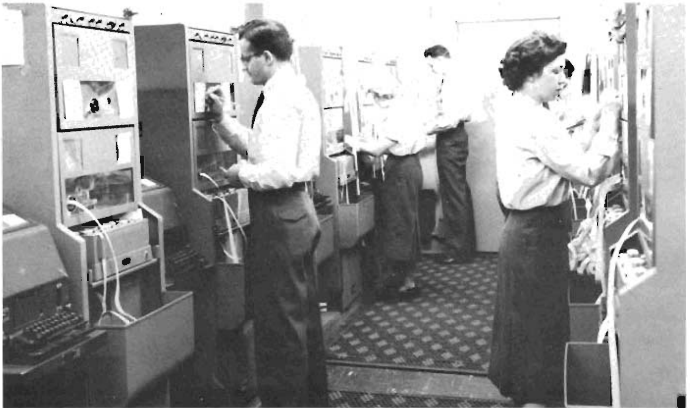
The Global Communications System, which was basically a radio system, was the first integrated communications system to span the world. Construction began in 1951. Pictured here is one of the system's torn-tape relay centers.
