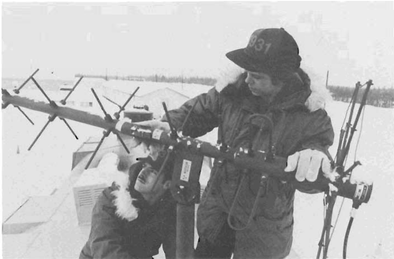
A1C Bill Lovins and Sgt Carol Burgwin, radio operations and maintenance specialists with the 1931st Communications Wing, adjust a satellite communications antenna during BRIM FROST 1985, a cold weather readiness exercise conducted every other year in Alaska.
