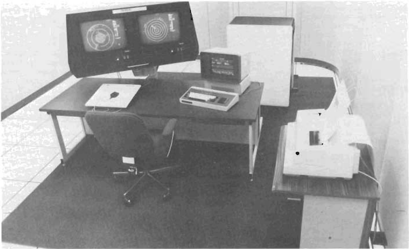
Next Generation Weather Radar was the name given to a joint agency program to acquire and deploy a new weather radar system. This new system would use doppler radars and computer technology, such as the prototype console pictured here, to allow better detection and measurement of storm severity, to improve warning accuracy, and to permit the automated exchange of weather radar data among federal agencies.
