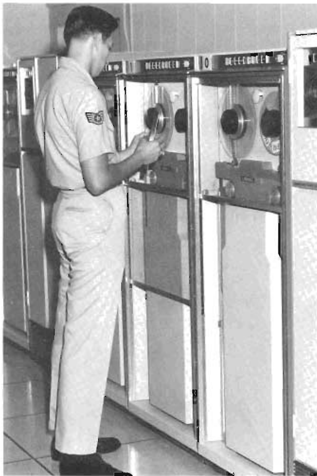
Information from this UNIVAC tape facility at Carswell AFB, Texas, provides a complete history of transmissions in the Automatic Digital Weather Switch.
