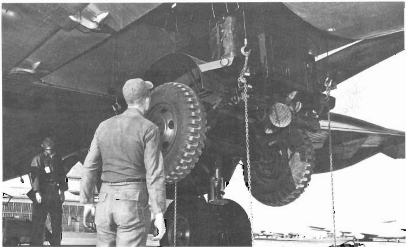
A mobile generator unit is loaded aboard a C-124 cargo transport aircraft at Tinker AFB, Oklahoma, for deployment to Alaska following the 1964 earthquake. The diesel-powered generator is part of the mobile control tower airlifted to Alaska to replace the damaged control tower at Elmendorf AFB.
