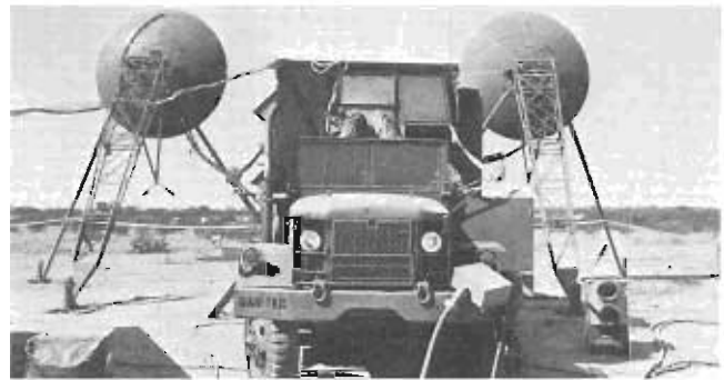
The AN/TRC-170 TRI-TAC radio tested by Detachment 1, 1815th Operational Test and Evaluation Squadron, could be set up and taken down quickly. This totally digital mobile radio was designed to provide cheaper and more accurate communications than the AN/TRC-97 radios. Since the AN/TRC-170 transmitter operated in the super high frequency range, the radio could be used in a line-of-sight mode or a tropospheric scatter mode.
