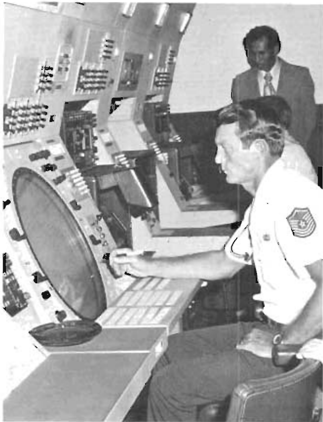
This air surveillance radar is used to take aircraft from one airport to another under radar control. Its range varies from seven to 240 miles.
