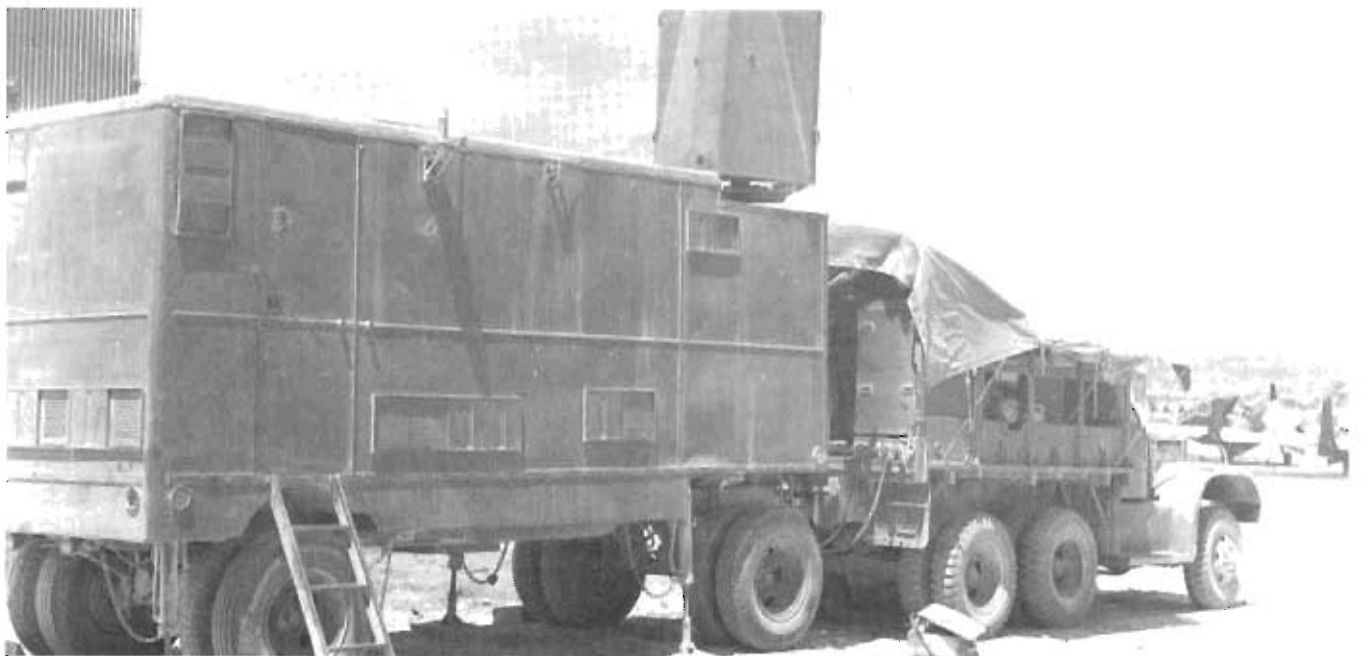
Ground control approach radar was probably the most significant navigational development during World War II. This new system, first employed by AACCS in England in the spring of 1944, enabled aircraft flying in extremely bad weather to land safely. An approaching aircraft could be sighted via radar through the heaviest fog when it was within a radius of 30 miles from the airfield. The aircraft could then be guided in by means of instructions from the control tower via radiotelephone. These two photographs display the exterior and interior of a ground control approach installation.
