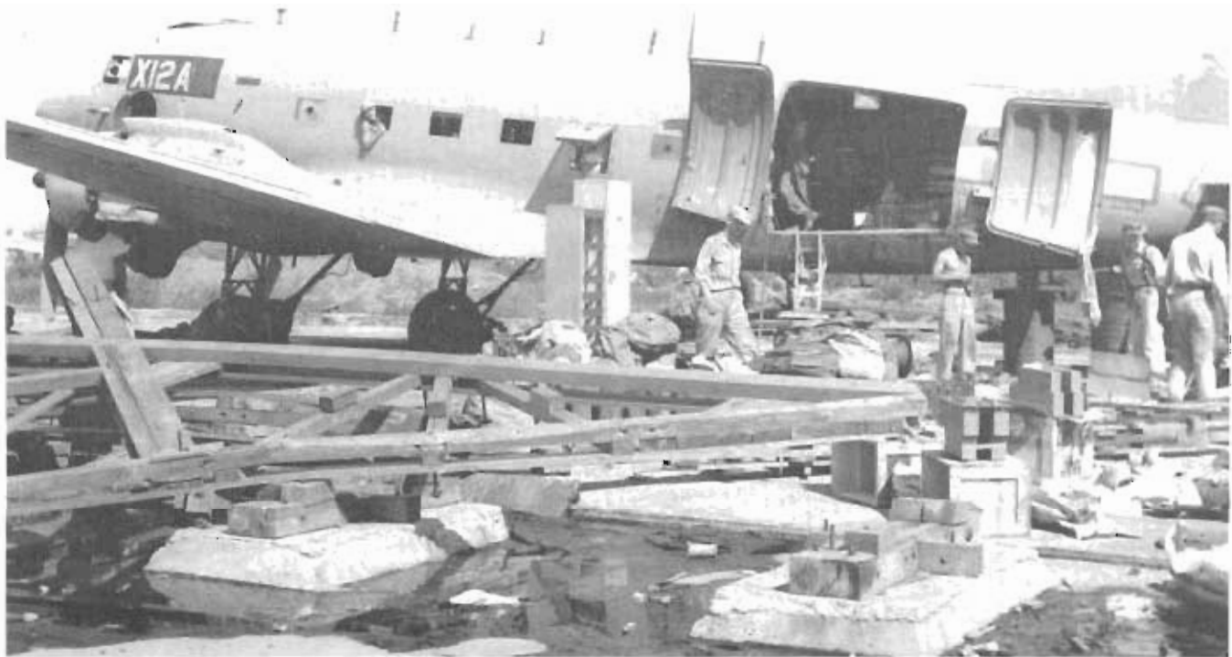
One hour after landing at Atsugi Airfield, near Tokyo, Japan, the AACS transmitter plane, a radio equipped C-47 (Gooney Bird), similar to the receiving station plane shown above, was on the air sending out signals to Okinawa. There was only one hitch in operations, when on the second day rains and motor traffic shorted out the five lines which ran to the receiver plane. Damage suffered by the field can be seen in the foreground.
