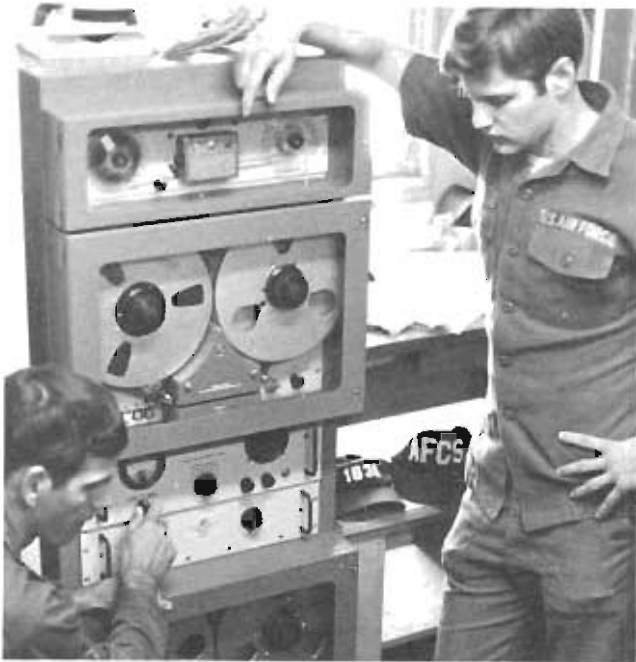
Two AFCS airmen check the AN/GSH-34 recorder installed as part of the control tower modernization program.
