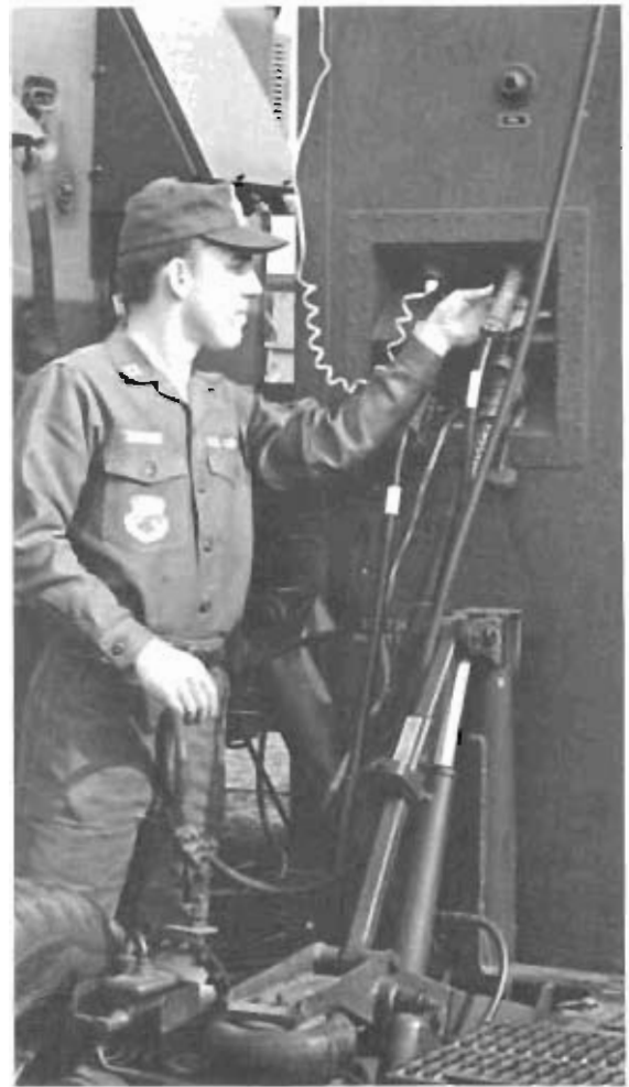
Constant checks are necessary to ensure the proper operation of mobile facilities. Here, an AFCS officer from the 2d Mobile Communications Group checks electrical power connections on a deployed AN/TSC-62 communications control van.
