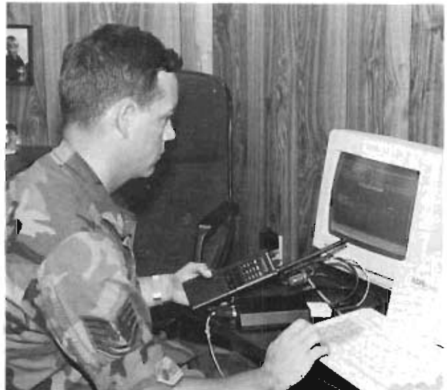
TSgt Gordon Smith, land mobile radio manager for Langley AFB, Virginia, programs one of the new portable radios with software loaded on a Z-248 computer. The unit acquired all the hardware and software needed to change frequencies in minutes rather than the months required to order crystals.
