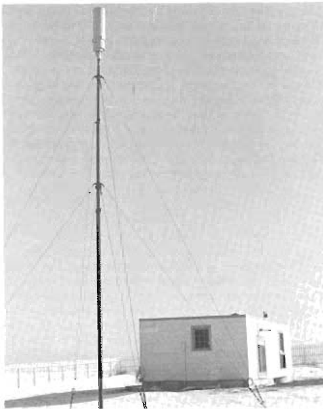
This AN/CRD-6 ultra frequency, crystal-controlled, automatic direction finder operated on one of 10 preset channels and could be remotely. Its range was limited to line of sight.
