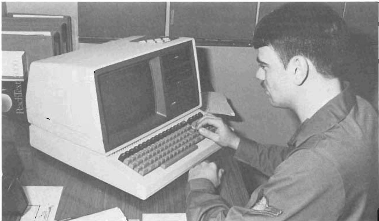
Airman Brian Turbide, operations administration clerk, 2192d Communications Squadron, prepares to take a communications security test on the new Z-100 microcomputer. These microcomputers were part of the office information system created by AFCC to change the way in which day-to-day business was conducted by automating many functions, such as word processing and records' management.
