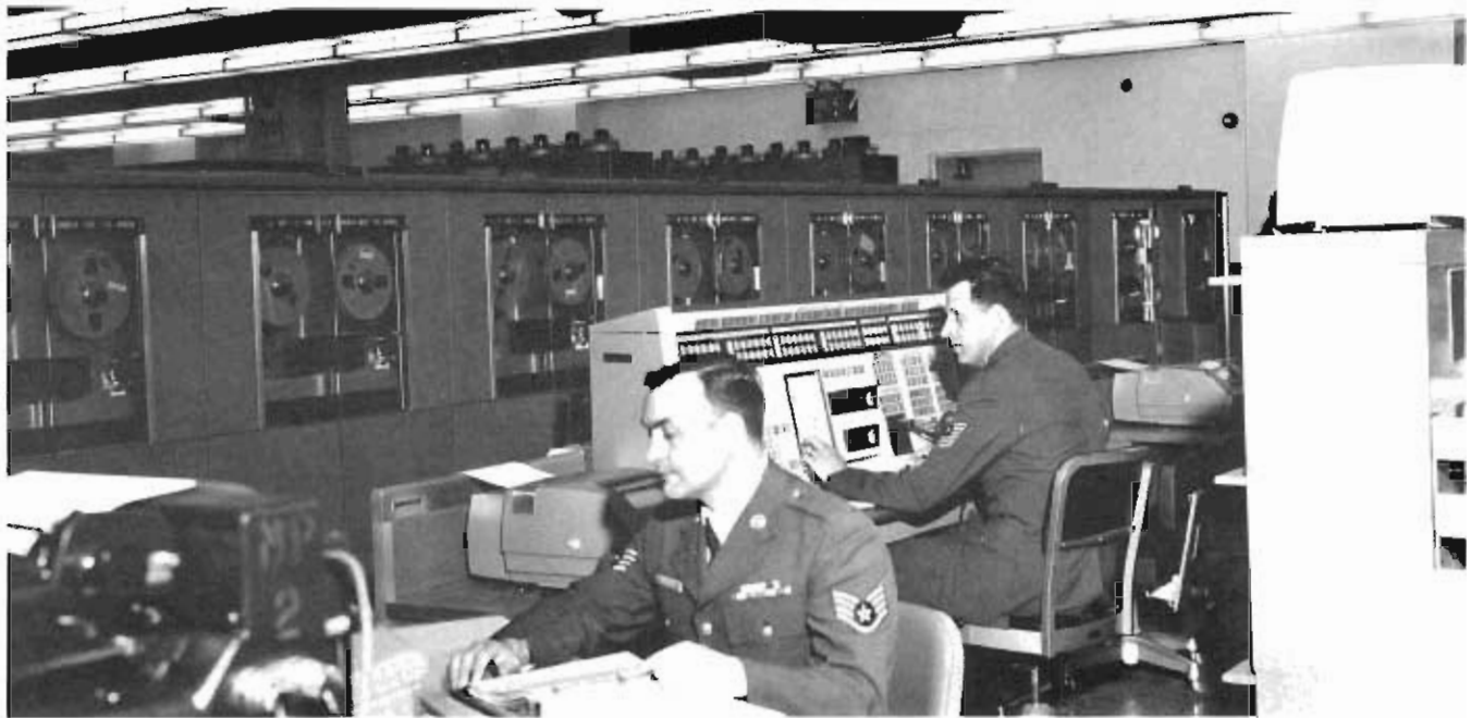
AFCC operated AUTODIN switching centers for the Air Force, like this one at Gentile AFS, Ohio. This completely automatic system is capable of handling any type of digital input teletype, data cards, or computer-to-computer information.
