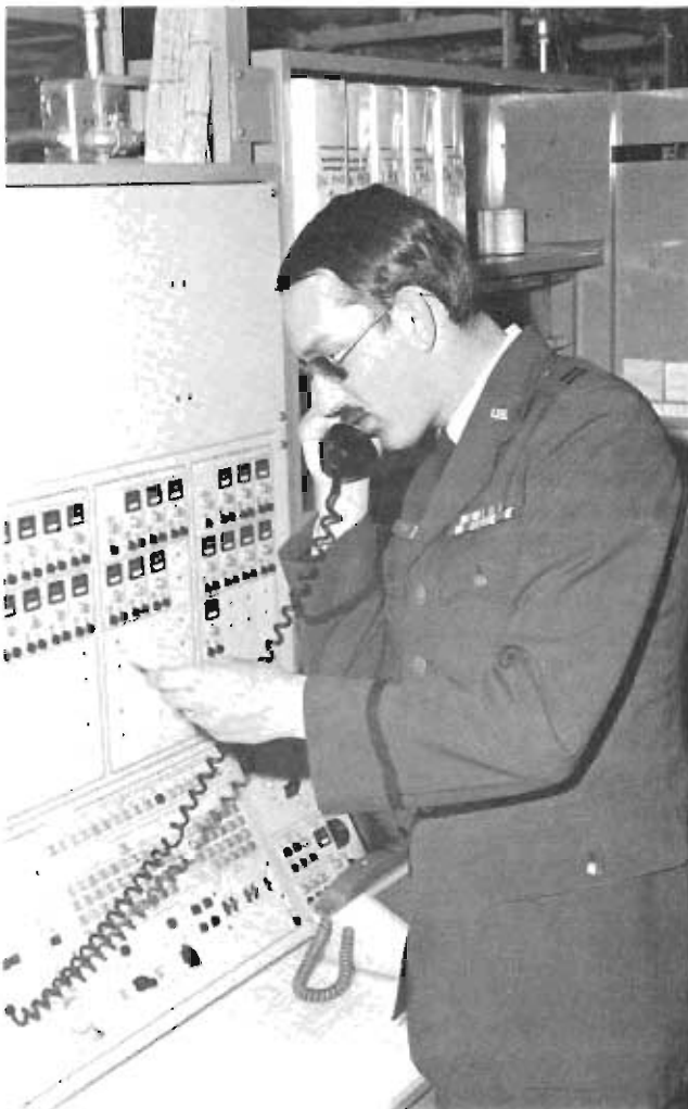
An AFCS officer interprets a card printout from the AUTOVON switch at Humosa, Spain.
