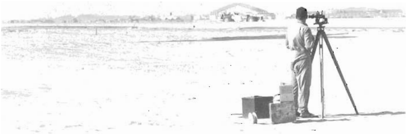
An AFCS sergeant measures the approach angle of an incoming aircraft during a check of the tactical air navigation unit at Chu Lai Marine Air Station, Vietnam.
