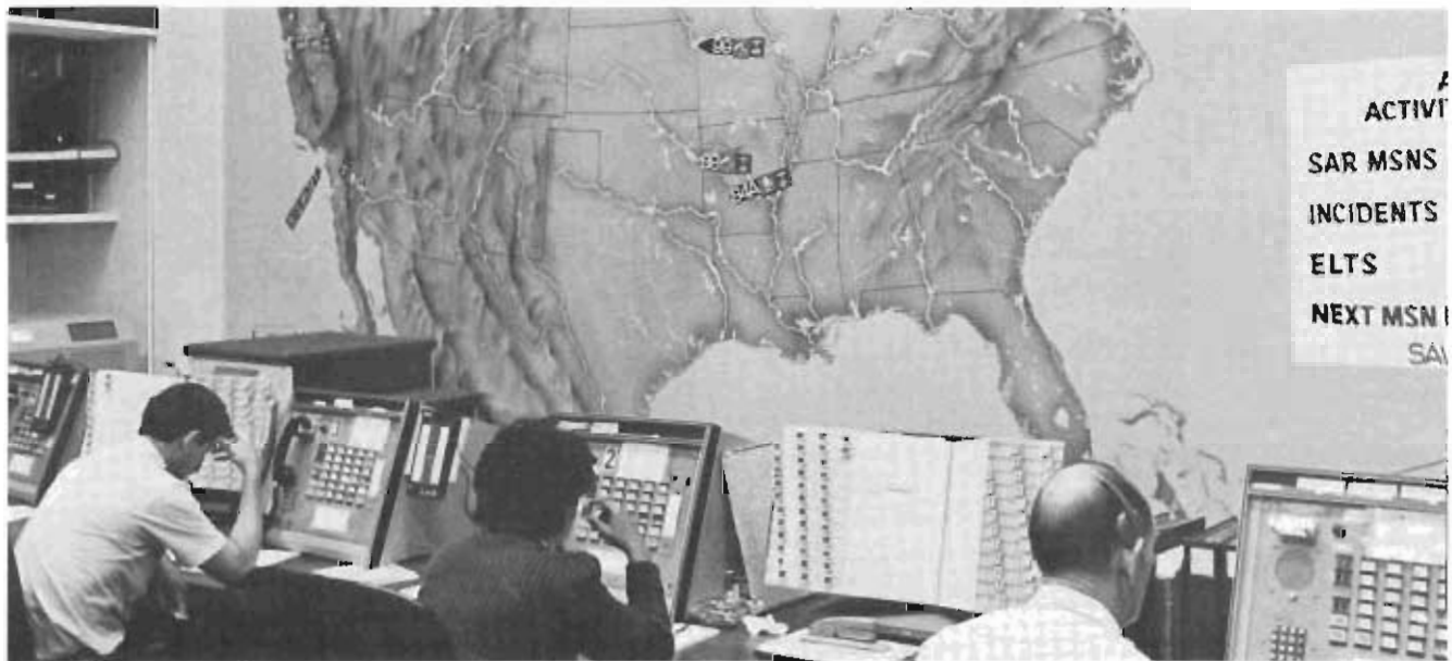
The Rescue Coordination Center of the Search and Rescue Satellite-Aided Tracking System at Scott AFB, Illinois, is staffed continuously. This system and its Soviet counterpart use satellites in low, near-polar orbits to search for aircraft and vessels in distress. AFCC's Airlift Communications Division's Automation Support Branch supports the effort at Scott by monitoring the communications lines and ensuring that data flows properly between the tracking system centers.
