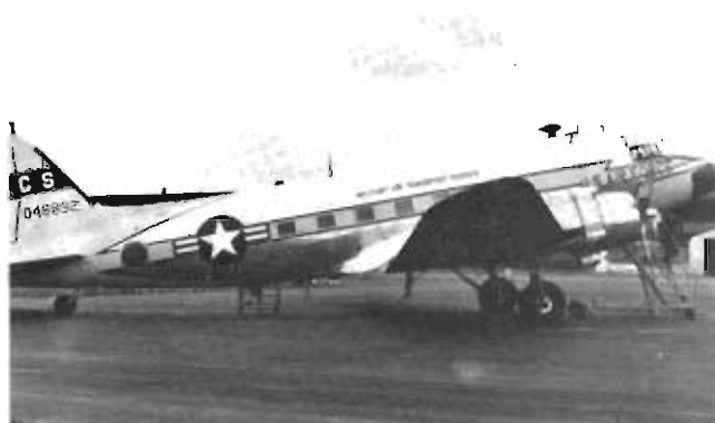
During the 1950's, AACS employed various types of specially configured aircraft to flight test and calibrate navigational aids and flight control facilities. The AC-47D pictured here remained active in the command's inventory until 1962.
