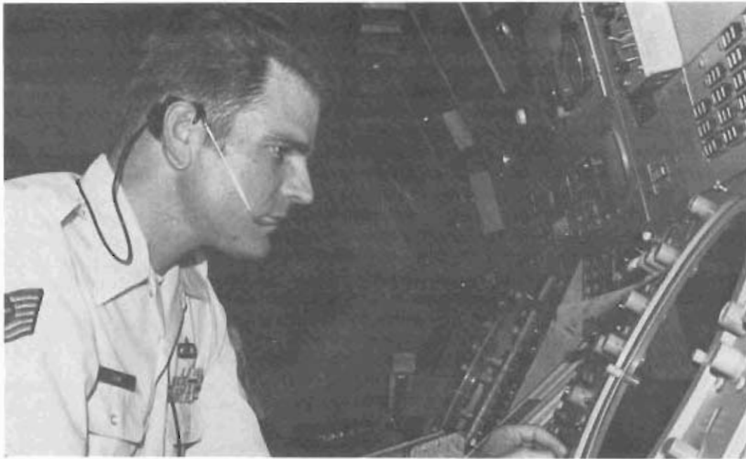
The OD-69 airport surveillance radar indicator with the AN/FPN-47 system at Scott AFB, Illinois. Scott AFB also has an AN/FPN-62 precision approach radar system.
