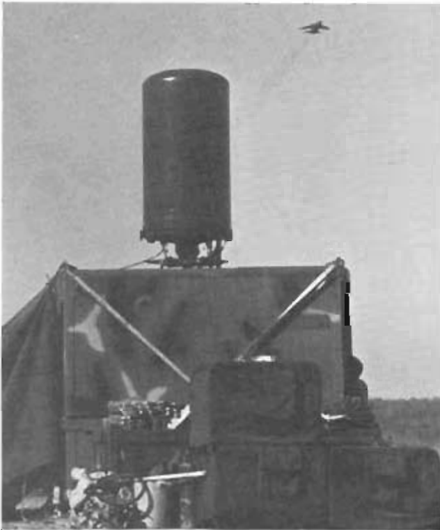
A portable AN/TRN-26B tactical TACAN is used to provide radio navigation to aircraft during a NATO exercise. The TACAN can provide bearing, identification, and distance information to as many as 100 aircraft simultaneously.
