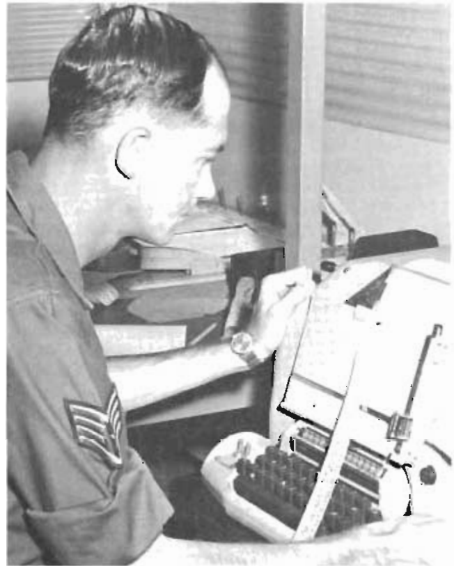
Introducing equipment that would transmit and receive messages in a variety of formats was one of the advanced features of the AUTODIN network. Here, an airman prepares a message on paper tape.
