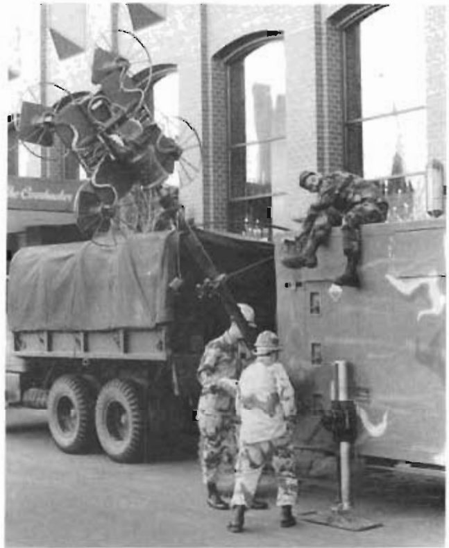
SSgt Tim Godwin (on top of van), SSgt Curt Tostie (foreground) and Amn Chris Winters attach the base of a satellite antenna to the AN/TSC-88 van.
