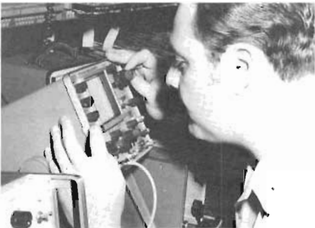
Sensitive telephone lines require special maintenance. Here, an officer from the 1835th Electronics Installation Squadron, Norton AFB, California, uses an oscilloscope to examine telephone lines for possible trouble or defects.
