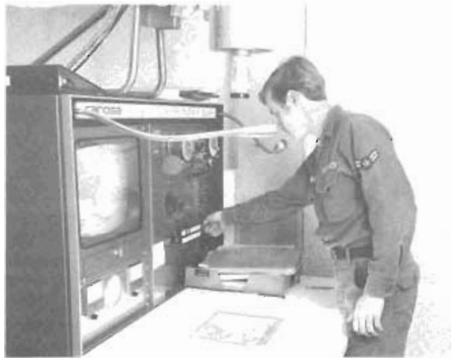
An AFCS airman adjusts the focus on a closed circuit television system in a base weather station.
