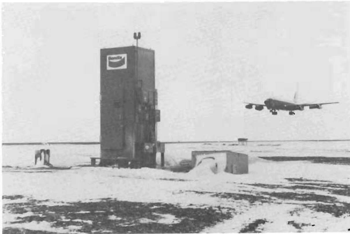
The microwave landing system at Shemya AFB, Alaska, would provide more accurate information than other landing systems.
