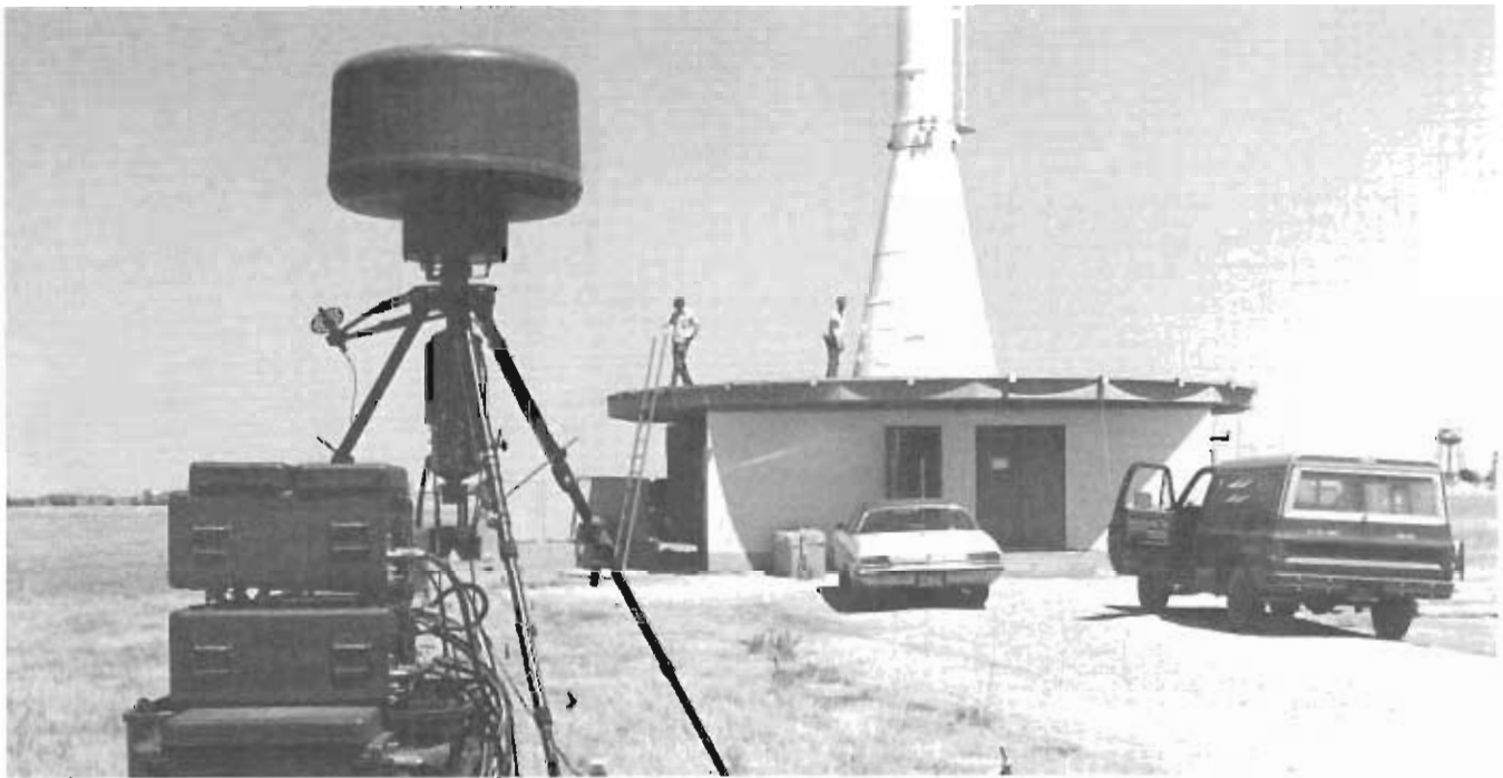
A mobile tactical air navigation unit sits near a permanent facility during repairs.
