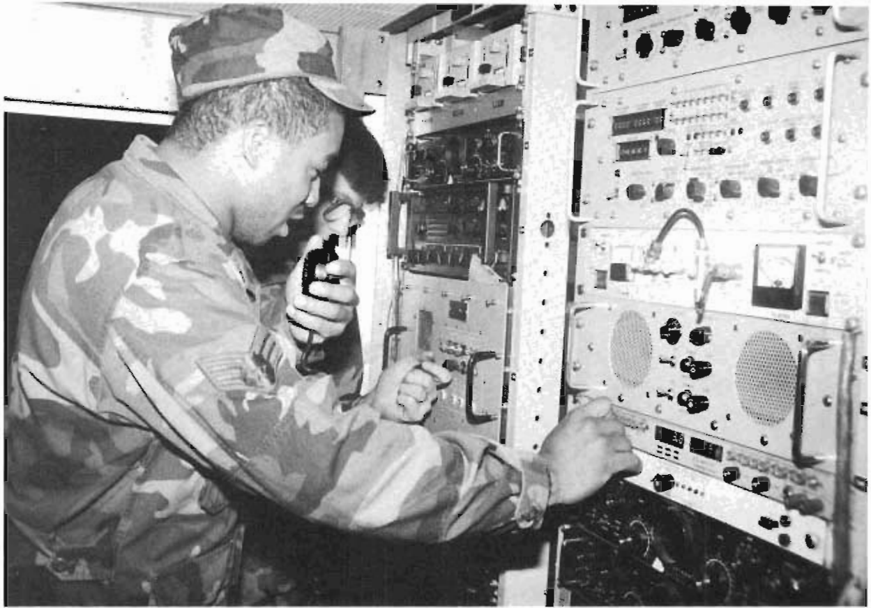
Sgt Keith Trawick, left, and Sgt Rick Chaples, both Quick Reaction Package technicians, manually change the settings of the high frequency radio in preparation for a data test with the Quick Reaction Vehicle.
