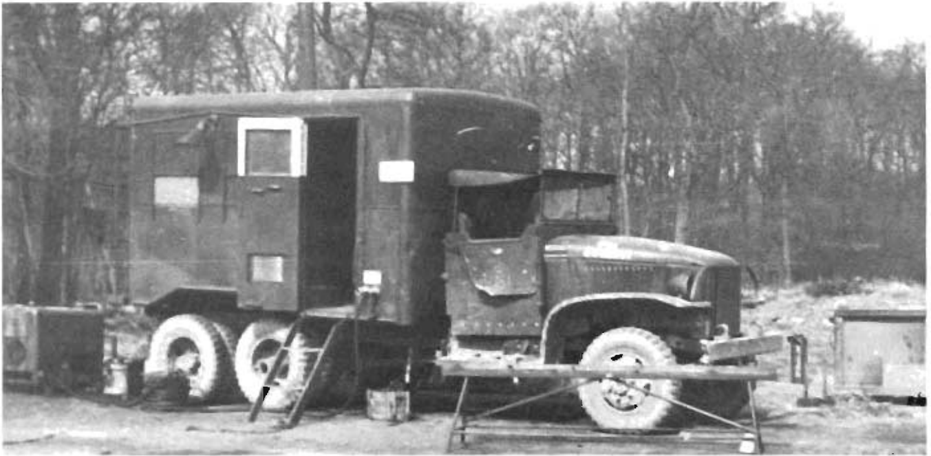
An AACCS mobile, low frequency transmitter was used during the Berlin Airlift as a homing beacon.
