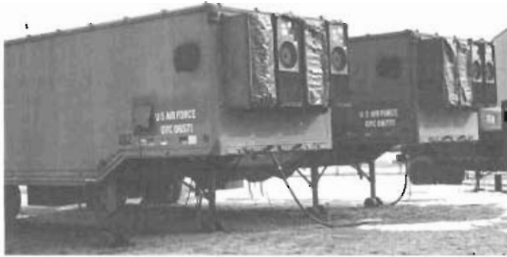
Mobile Digital Subscriber Terminal Equipment provides message service when system improvements or combat exercises preclude the use of fixed AUTODIN facilities.
