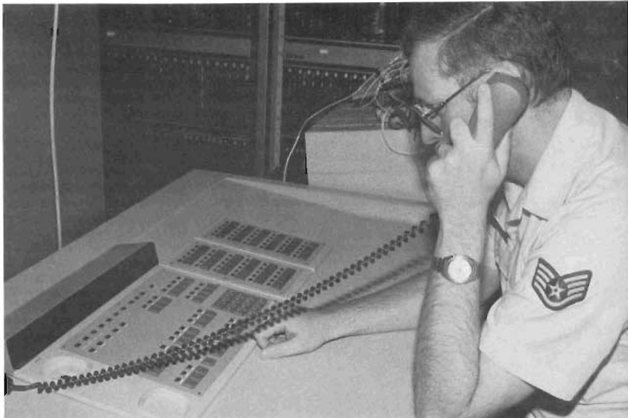
SSgt William C. Mehrhoff, 2134th Communications Squadron, NCOIC of telephone operations at Sembach AB, Germany, checks out one of the new terminals that will be installed to program the European Telephone System. This system was the European component of AFCC's Scope Dial program, a world-wide project to modernize the telephone systems at Air Force bases by using state-of-the-art equipment. The system at Sembach was only the second of its kind to be installed at a US Air Force location in Europe.
