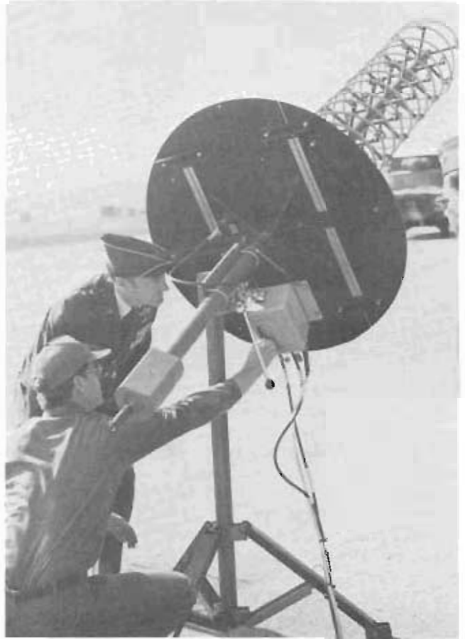
A1C Timothy Cash of the Satellite Communications Branch, 3d Combat Communications Group, demonstrates the TSC-102 system, detailing its antenna operations, to Maj Gen William G. MacLaren, Jr.
