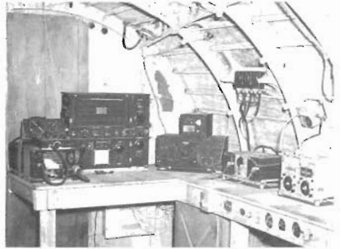
Interior shot of the radio installations in the C-46 fuselage. Equipment includes command transmitters and receivers and a BC-348 high frequency receiver.
