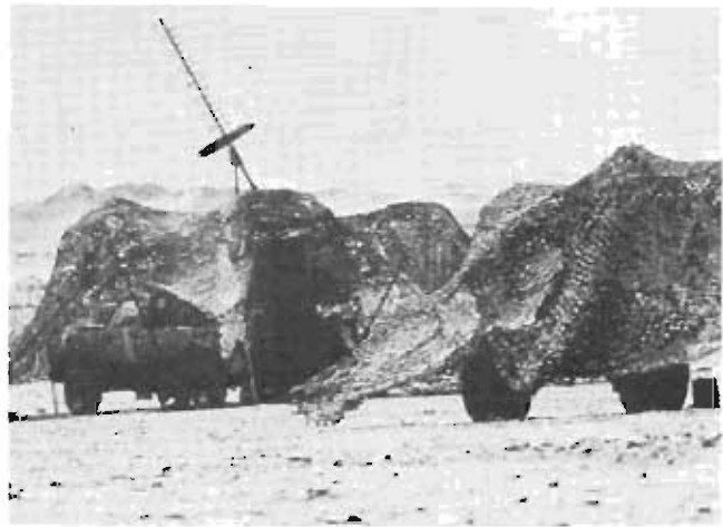
Camouflage netting helps conceal this mobile satellite terminal and helical antenna.
