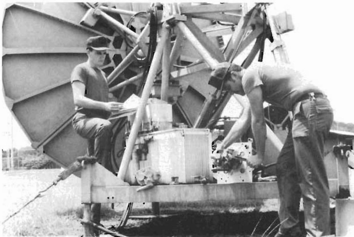
MSgt Larry Flohaug, left, puts filters on a new hydraulic system pump for the Mark IV transportable weather terminal, as Sgt Ron J. McNally, space systems equipment technician, reads off the technical order checklist.
