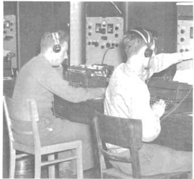
Point-to-point communications from one station to another was an important part of AACS's job. Sometimes messages were sent by Morse code over radio (known as continuous wave), teletype, or by radioteletype. A variety of messages could be transmitted by point-to-point communications, but the primary uses were to relay information on the movement of aircraft or weather conditions. These AACS men in Berlin are receiving continuous wave (CW) transmission.
