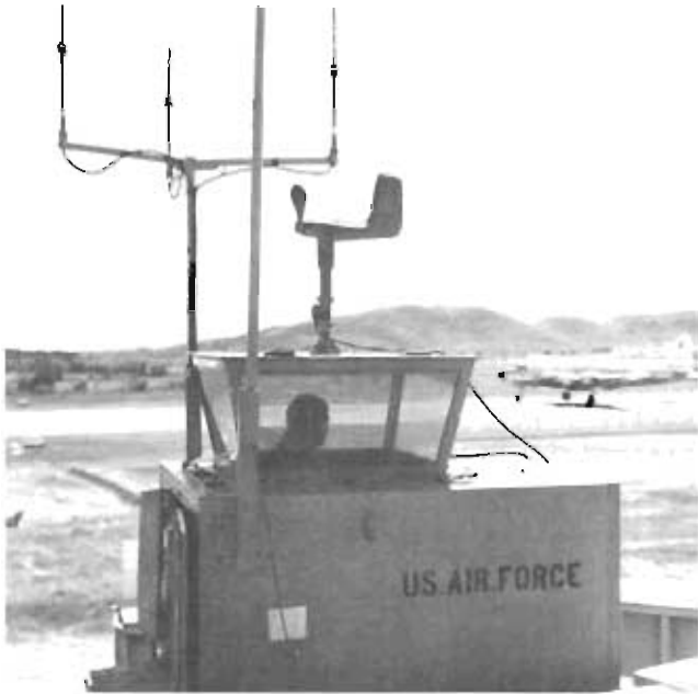
A mobile runway supervisory unit directs aircraft at Phu Cat AB, South Vietnam, as a C-54 takes off in the background.
