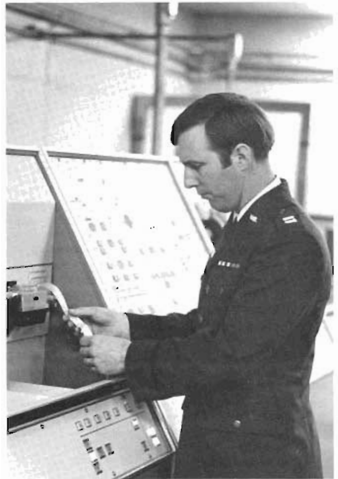
The chief of operations for the 2187th Communications Group at Aviano, Italy, checks tapes from the electronically controlled Digital Subscriber Terminal Equipment.
