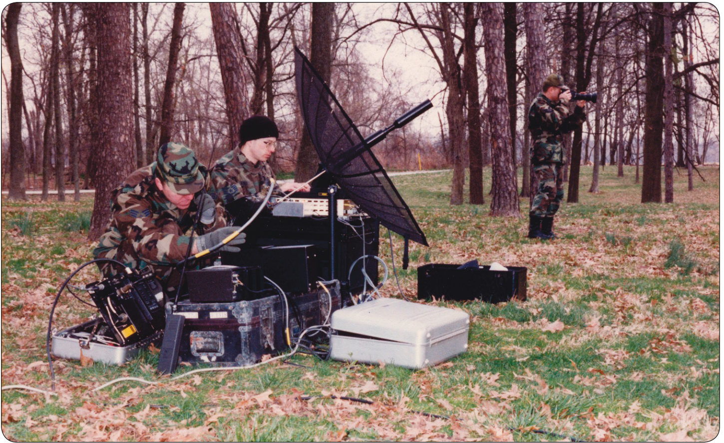
Two AFC4A Hammer ACE team members setting up the LSSC-300 terminal and portable satellite antenna during a training exercise at Scott AFB during the 1990s.
