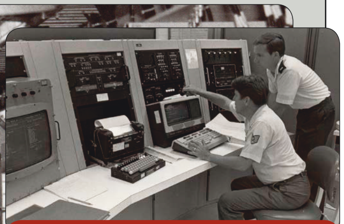
An AFSATCOM programmer, Tech. Sgt. Otis Smith, operates the AFSATCOM simulator while 2nd Lt. Rick Mahoney, Test Analyst watches. The simulator was capable of reproducing the necessary inputs and outputs that show real-world choices that can be handled by radio receiver, transmitter, and satellite equipment, Tinker AFB, Oklahoma, Aug. 12, 1983.
