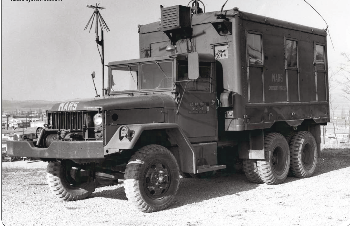
Truck-mounted emergency Military Affiliate (Auxiliary) Radio System station.
