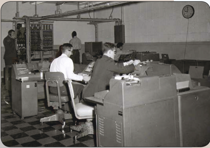
Pre AUTODIN view of a data communications manual relay facility, late 1950s early 1960s.
