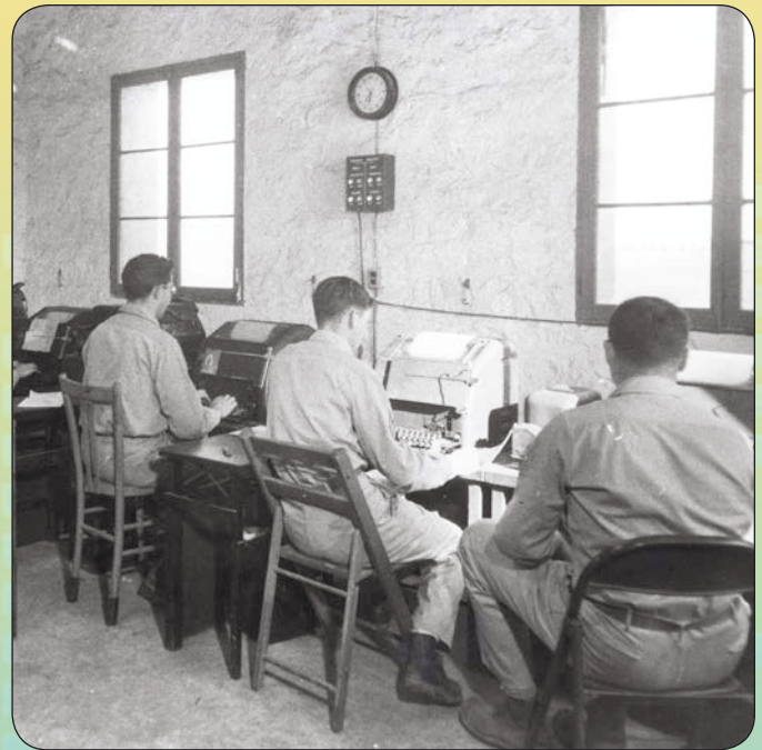
TELETYPE COMMUNICATIONS: Perforated tapes for transmission hang on the left side of the teletype room as members of the 19th Army Airways Communications System Squadron use model 30 and 36 teletypes to send communications out.
