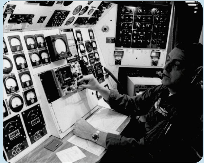
Inside view of one of Air Force Communications Command's C-140 "Jet Star" with Chief Master Sgt. Tony Haus working the flight inspection equipment console.
