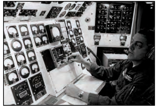
Inside view of an AFCC C-140 JetStar with CMSgt Tony Haus working the flight inspection equipment console. (Courtesy of AFNIC History Office)
