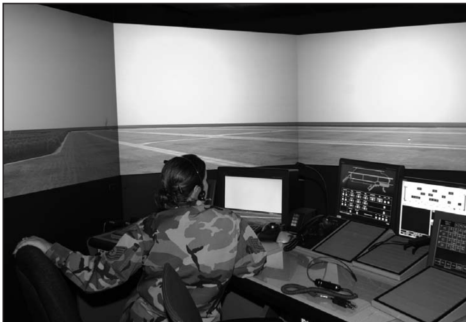
TSgt Wendi Drusch scans the graphically-generated airfield during a Tower Simulator System (TSS) training scenario. Installed in 2005, the $800,000 TSS simulates the actual Columbus AFB airfield environment on its six screens and features voice-recognition software that responds to controller instructions. One trainer can simultaneously train three controllers while manipulating traffic intensity, weather, airfield lighting, emergency conditions and pilot responses.
