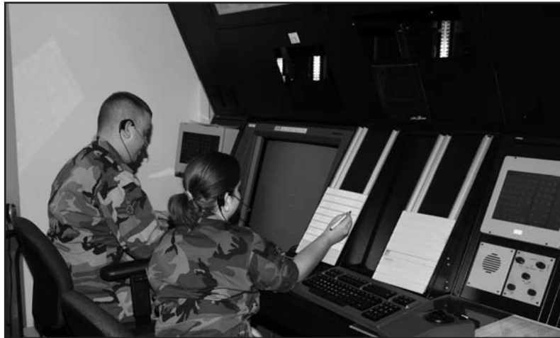
A1C Justin Caldwell & A1C Leslie Rangel training on ATCoach simulator, ATCoach was procured in conjunction with the Standard Terminal Automation Replacement System (STARS) and can be used as a simulator or as a live scope.
