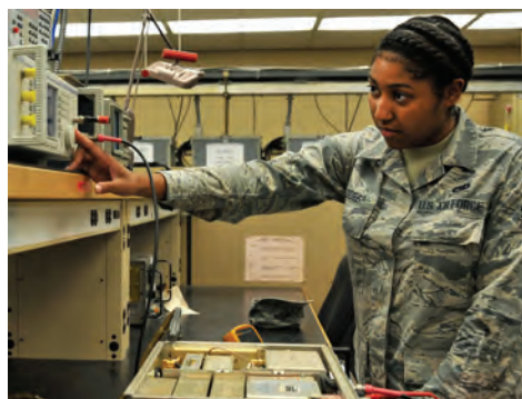
A1C Darricka Sides, 20th OSS airfield systems technician, sets up a signal generator for radio receiver tuning at Shaw AFB, S.C. (Air Force photo by A1C Kathryn R.C. Reaves)
