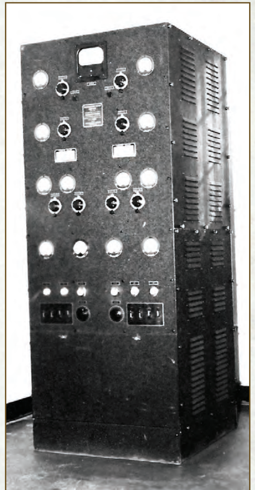
1200 W LF PanAm transmitter used as homer
