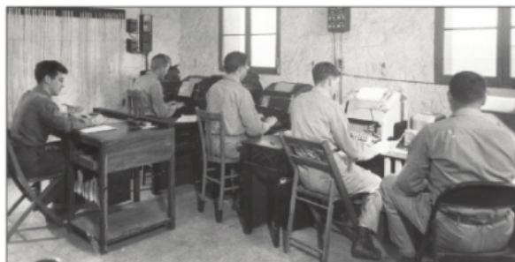
Perforated tapes for transmission hang on the left side of the teletype room as members of the 19th Army Airways Communications System Squadron use model 30 and 36 teletypes to send communications.
