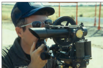
An 1866th Facility Checking Squadron flight inspection technician talks to the flight check pilot while looking at the approaching flight check aircraft through a theodolite.
