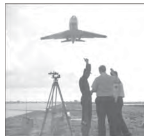
A flight inspection technician gives the aircrew in the AFCC C-140 "Jet Star" a thumbs up indicating a successful glide slope run. Note the theodolite set up beside the runway to record flight inspection data.
